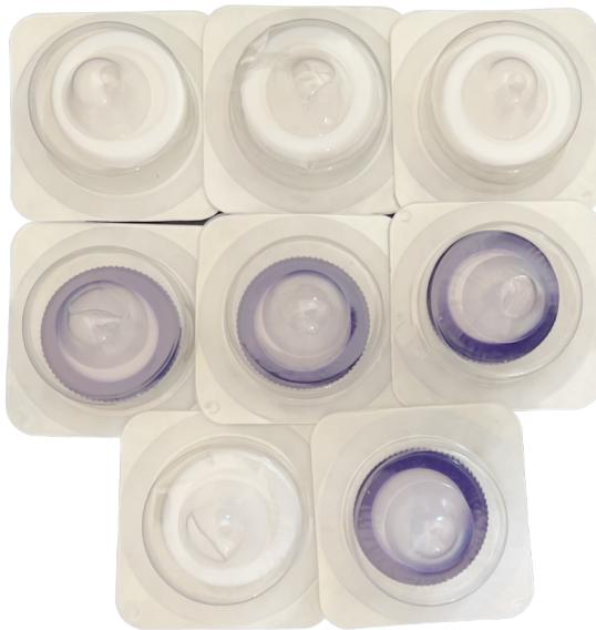
MQ Syringe Filters are pre-sterilized by gamma rays, individually wrapped and for single use. They ensure high purity of filtrate because of their non-pyrogenic, low extractables and surfactant-free material. They have extreme-low protein binding <1.5% (PES), excellent throughput, for faster filtration and more process volume.
